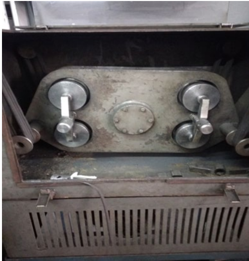
Fig. 1 Photographs of laboratory research: c – cylindrical mill on elastic suspensions;
