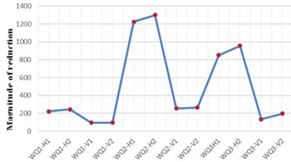
Figure 8: The pattern of permeability changes observed in limestone samples under depressurization condition.
